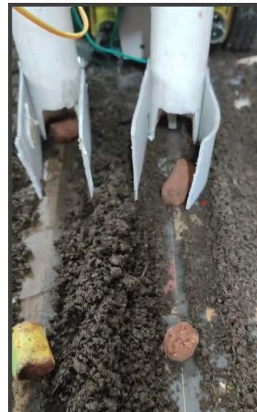
Fig 8. Furrow creation by T-splitters
