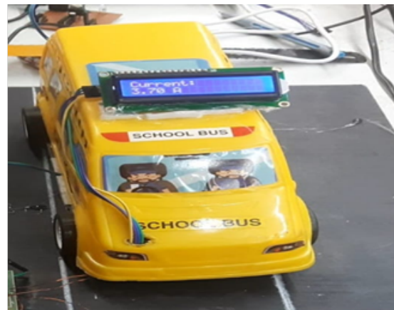
Fig 4. Current output readings at minimum coil distances using ACS712 sensor
