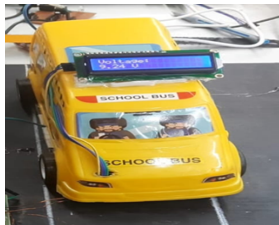
Fig 5. Output Voltage readings from receiver coil at minimum air gaps
