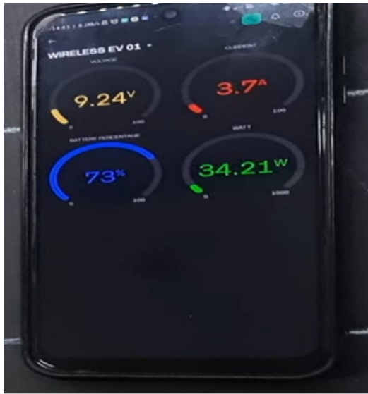
Fig 6. Blynk IOT app displaying real-time voltage and current from ESP32
