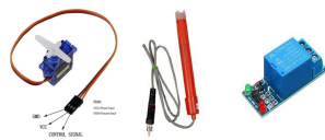
Fig 3. Servo Motor sensor Relay water pump
