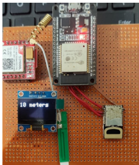
Fig 6. Anchor uses UWB to locate TAG
