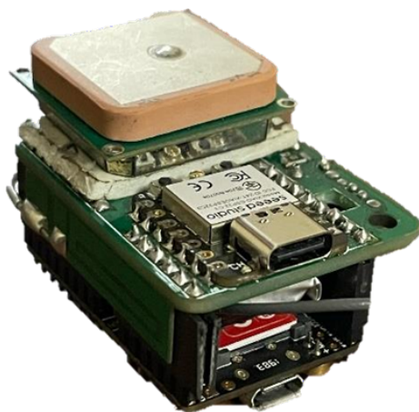
Fig 7. Tag using GPS and GSM to send location to user
