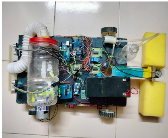
Fig 3. Structure of multi surface floor cleaning robot
